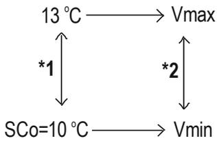
For **compressor operation** (parameter IAO = 0), 10 $^{\circ}$ C corresponds to Vmin and 13 $^{\circ}$ C corresponds to Vmax
