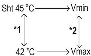
For **compressor operation** (parameter IAO = 0), 45 $^{\circ}$ C corresponds to Vmin and 42 $^{\circ}$ C corresponds to Vmax
