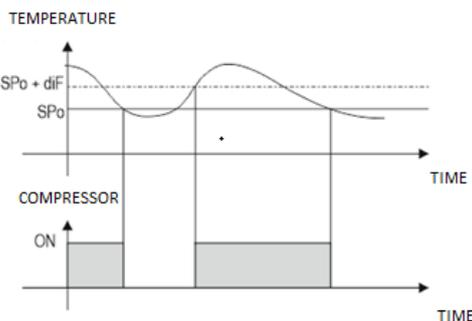
The regulation is performed according to the temperature measured by the thermostat probe with a positive differential(diF) from the set point. If the temperature increases and reaches set point (SPo) plus differential the compressor is started and then turned off when the temperature reaches the set point (SPo) value again. In case of fault in the thermostat probe the start and stop of the compressor are timed through parameter "**Cf**".
