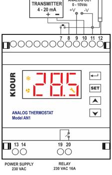
ATTENTION: No other device than the transmitter must be connected to terminal No. 8.
